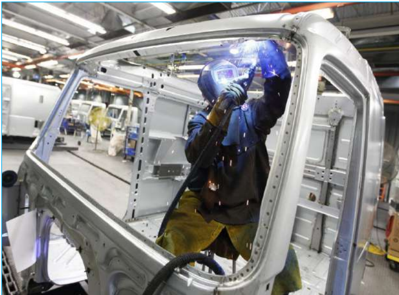
Fig. 18.2.3.5: A worker welds a cab frame in Dublin, Virginia
